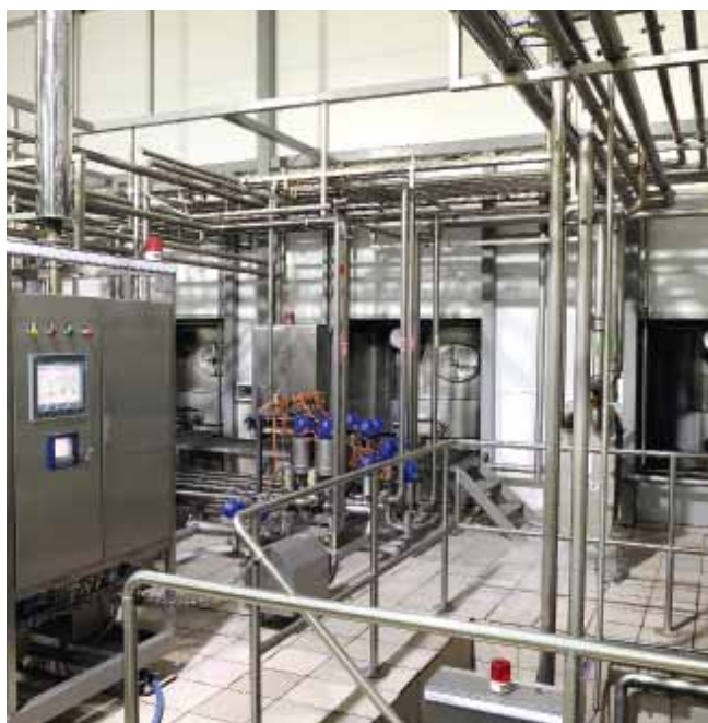
Moloko Dairy milk reception plant upgraded with Alfa Laval Unique SSV valves, LKB valves, ThinkTop valve sensing and control units, Solid C and LKH centrifugal pumps and energy-efficient agitators.
