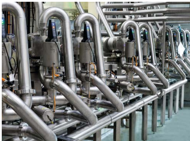
The new Kompak pigging system features Alfa Laval OptiLobe rotary pumps, LKB butterfly valves, IndiTop valve position indicators and fittings for straightforward operational reliability.
