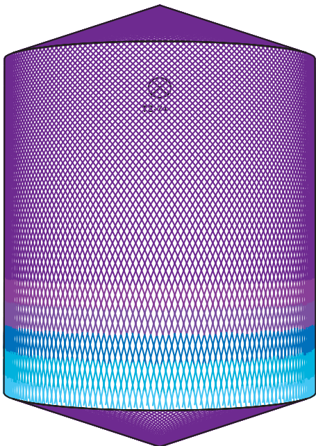
D5m H6m, Toftejorg TZ-74, 4 x ø 7 mm, 0% Time = 19 min., Water consumption = 5408 l (1429 gallon)
