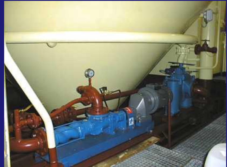
Eccentric screw pump. (for discharging the mud-tank)
