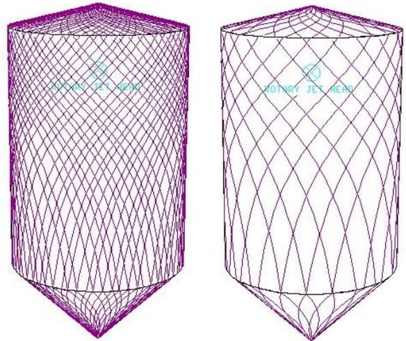
Figure 4. Simulation showing a standard burst coverage using a standard rotary jet head (left) and a burst sequence using a burst cleaning nozzle type Alfa Laval Rotary Jet Head (right). In both cases, the tanks are fully wetted, but the burst cleaning sequence provides fast wetting of the tank using a significantly reduced amount of cleaning fluids.
